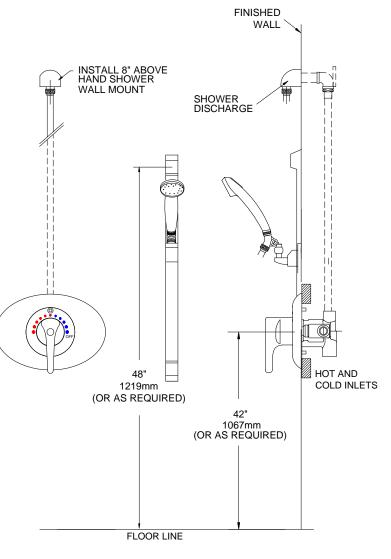
All Leonard Model 7600 Thermostatic Shower Valves have limitations. Please keep in mind that per the ASSE 1016-2011 Performance Standard, Harmonized along with ASME and CSA, it dictates inlet conditions of equal pressures, 45 PSI on both Hot and Cold Inlets, in addition to a Hot supply temperature range of 140 deg F-180 deg F. Significant deviations from those conditions stated above will alter performance expectations.
